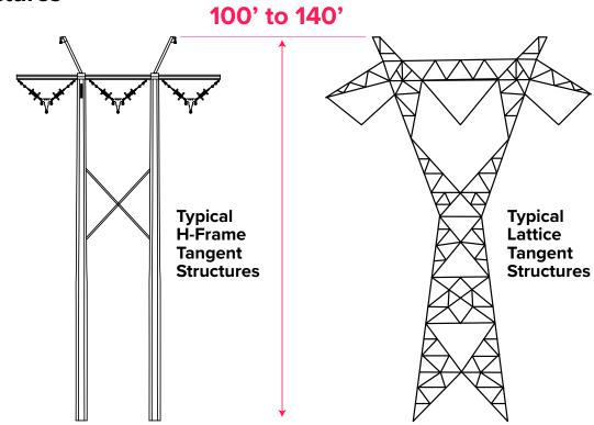
Typical structure shown. Structures along the route are subject to change based upon location and design requirements.
